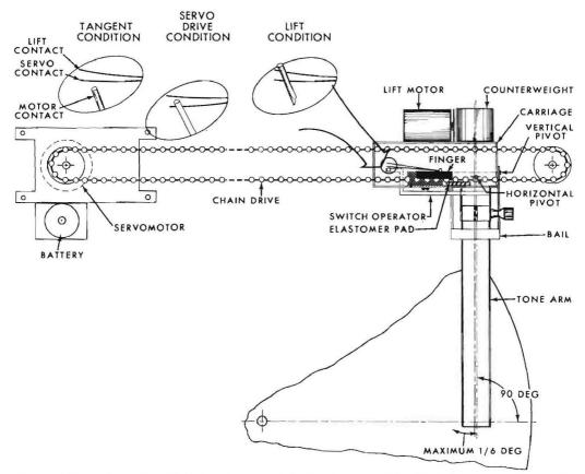
Tone-arm linkage closes drive circuit when tone arm pivots from tangent position. Gimballed tone arm is supported in carriage on nylon rollers. Chain drive, connected to servomotor through 500:1 gear reduction, advances arm. Arm grips chain between metal finger and elastomer pad when arm is placed in the playing position.
